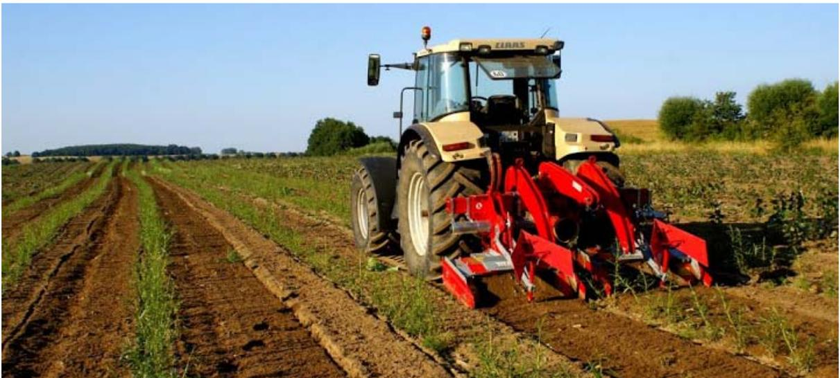
**Figure 10: Mechanical weed control with a tractor mounted rototiller from Badalini**
