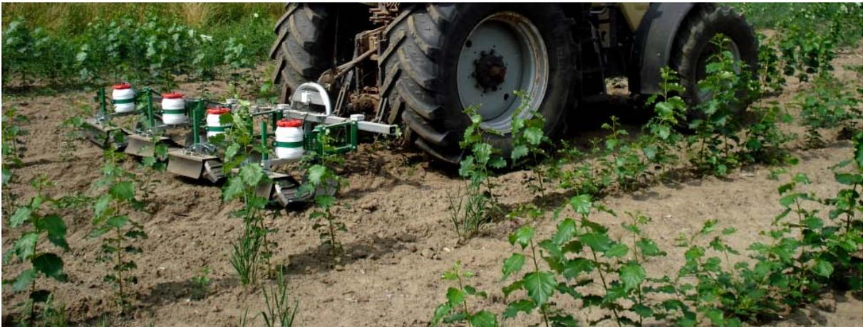
**Figure 11: Chemical weed control with shielded spraying system**
