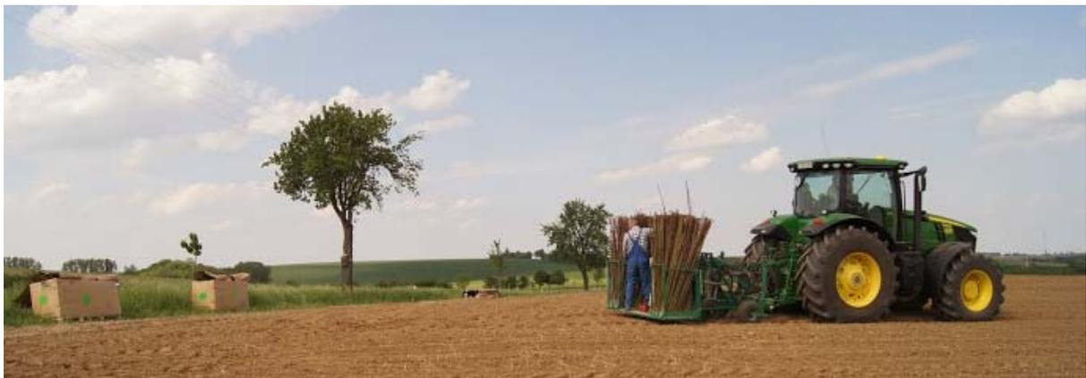
**Figure 9: Planting poplar with the “Step-planter” (planting material is delivered in boxes to the field side)**
